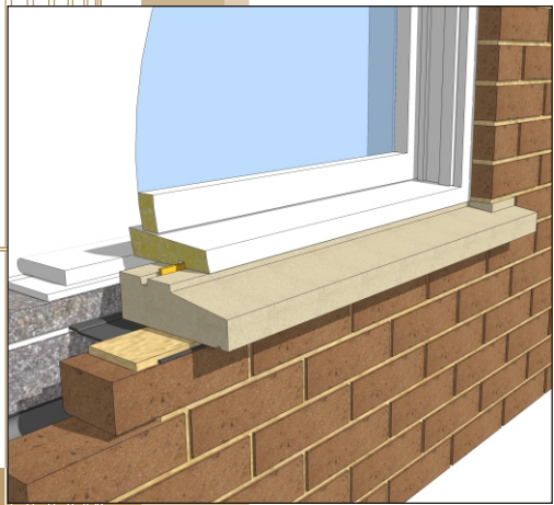
Typical installation detail
